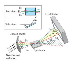
are the same for all the directions, the momentum transfer continuously varies because the X-ray energy (wavelength) changes as a function of direction. The normalized horizontal intensity distribution behind the specimen represents the CTR scattering profile.
